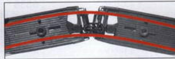
On curves the slot guide mechanism creates a larger gap between the wagons, so that the buffers do not lock.
